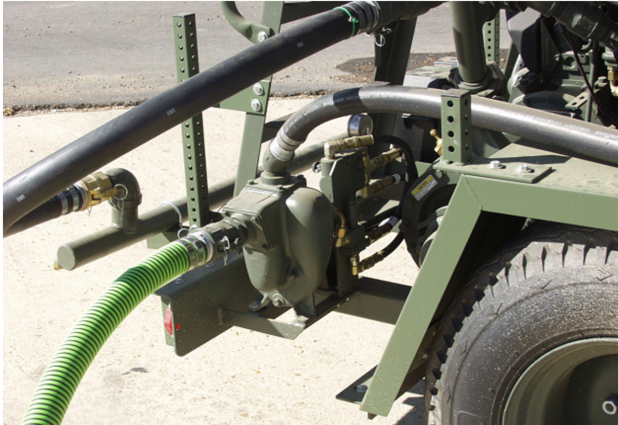
Photo 16. Filling HydroSeeder from storage container using onboard hydrostatic pump
