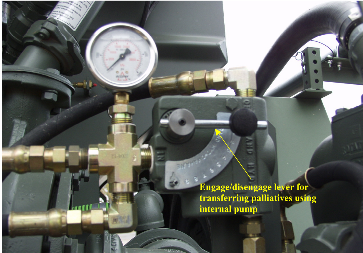
Photo 17. Hydraulic suction pump engagement lever on Finn HydroSeeder
