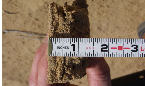
Photo 8. Desired crust thickness for emulsions to prevent FOD
