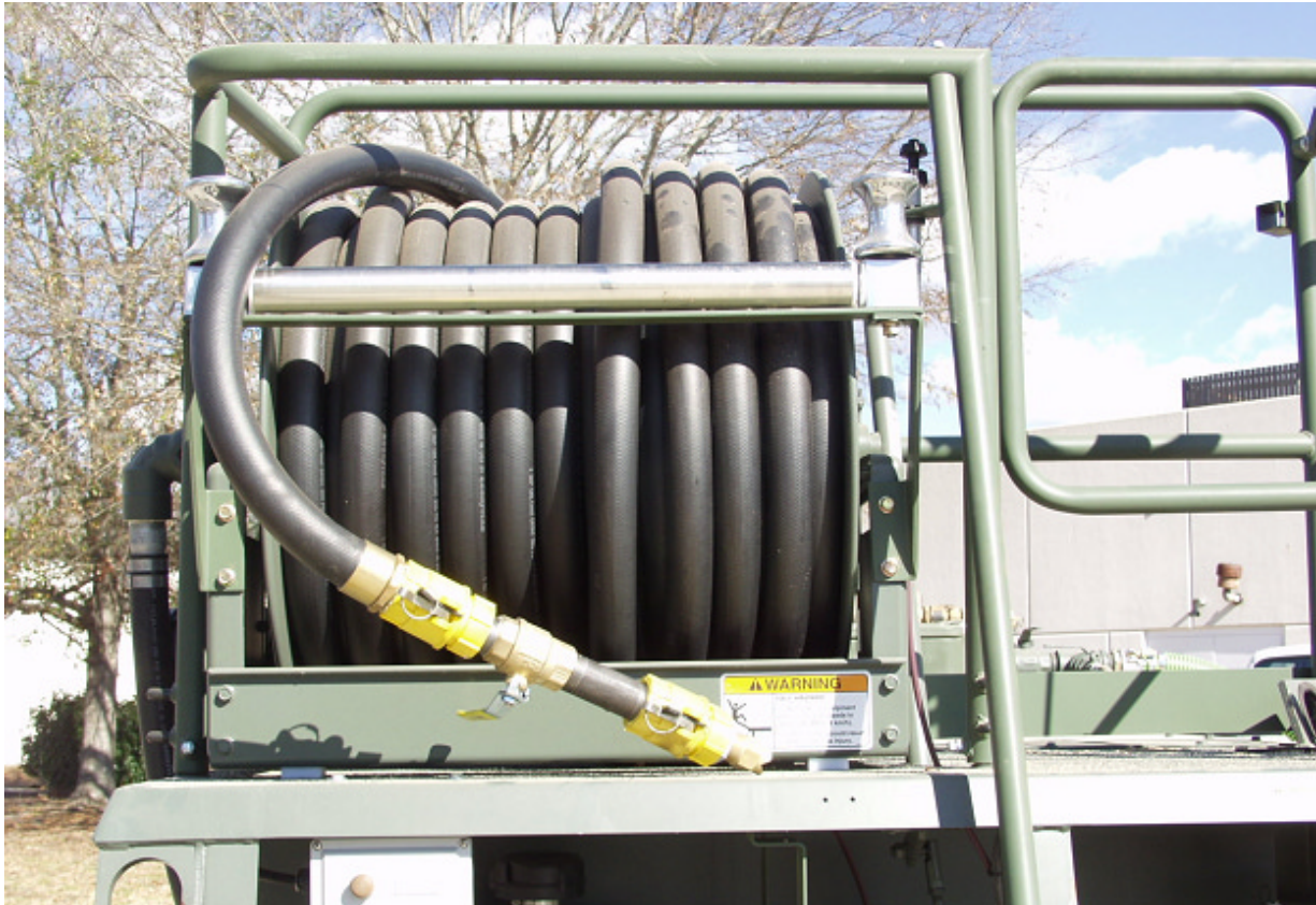
Photo 20. 200-ft hose with electric reel for multiple-use palliative distribution
