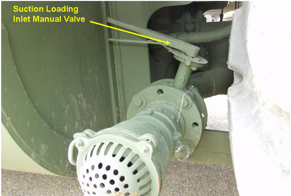
Photo 27. Suction loading inlet manual valve.
