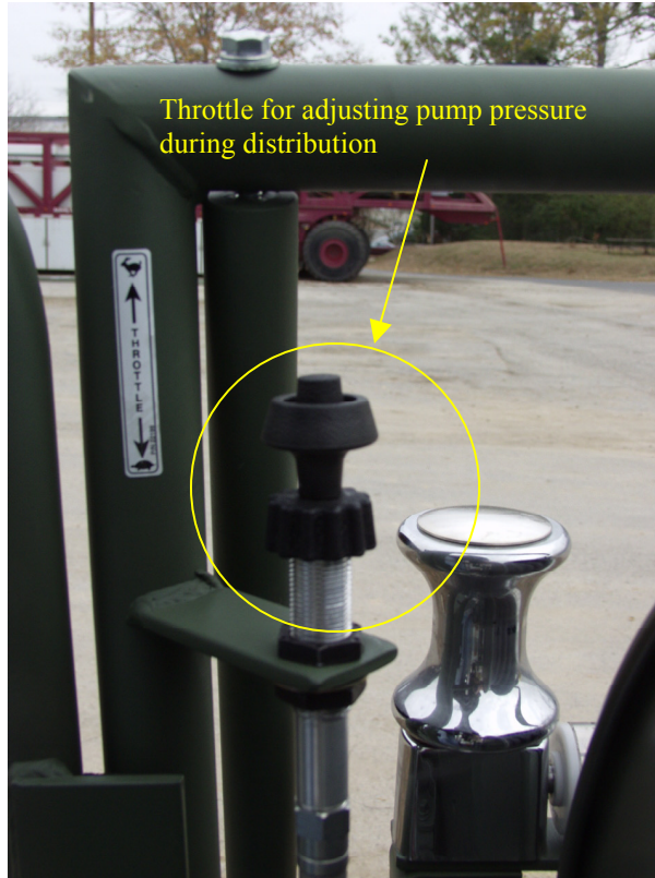
Photo 22. Engine throttle for Finn HydroSeeder located by tower gun
